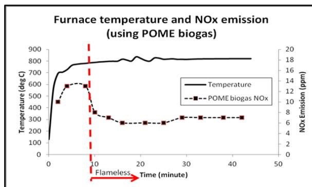
Figure 3 Furnace temperature and NO<sub>x</sub> emission for conventional flame (left of red line) and flameless combustion of POME biogas (right of red line)
