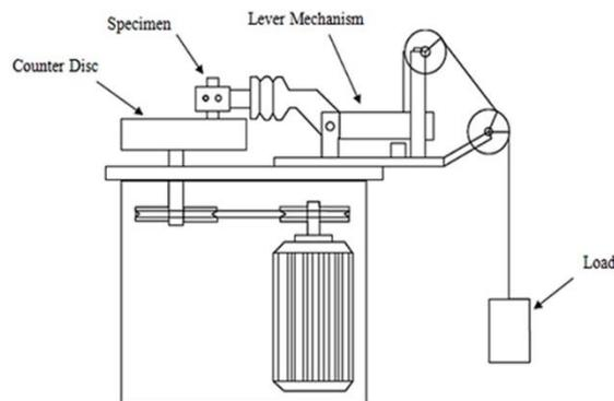
Figure 1 Schematic diagram of a pin-on-disc tribometer
