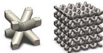
Figure 1 BCC single unit cell and one complete lattice structure block
