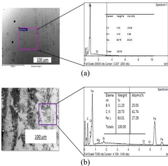
Figure 4 SEM micrograph and EDX spectrum for (a) 0.0 vol.% and (b) 0.2 vol.% of hBN concentration.
