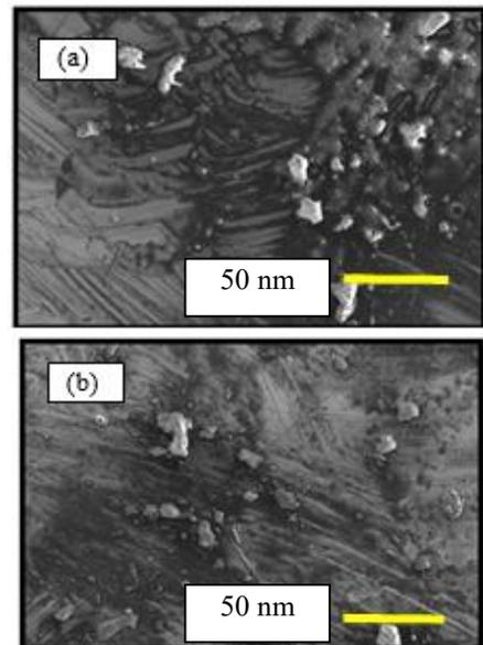
Figure 4 SEM micrograph of (a) 0.5 vol.% and (b) 1.0 vol.% of hBN concentration
