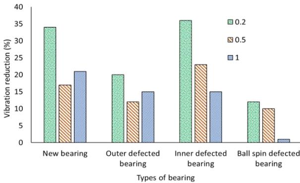
Figure 3 the reduction of vibration amplitude in ball bearing mixed lubricant
