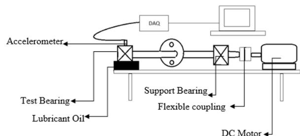
Figure 1 The vibration experimental test rig
