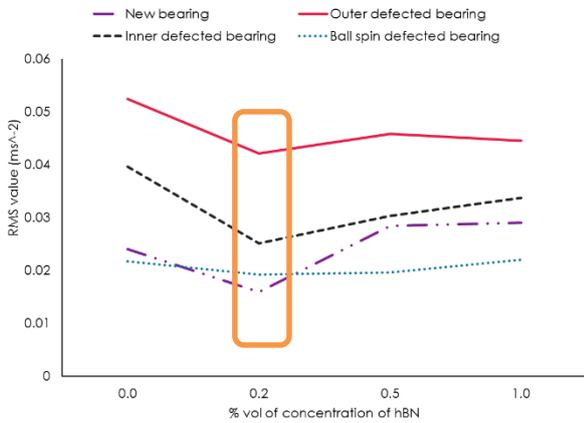
Figure 2 Vibration amplitude for new and defected bearings
