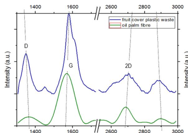
Figure 6 Raman spectra for carbon growth on Cu substrate from fruit cover plastic waste and oil palm fibre sources
