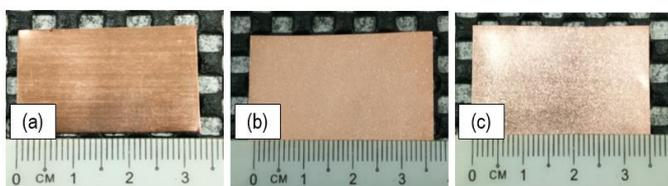
Figure 4 The surface image of (a) a pure copper, (b) carbon grown from fruit cover plastic waste, and (c) oil palm fibre source
