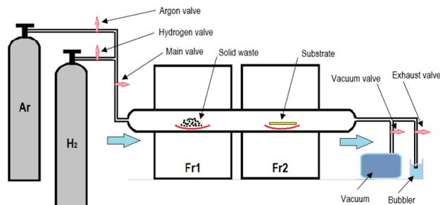
Figure 2 Schematic diagram for CVD process
