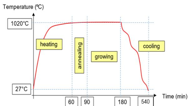
Figure 3 Heating, cooling, growing and cooling graph of the CVD process
