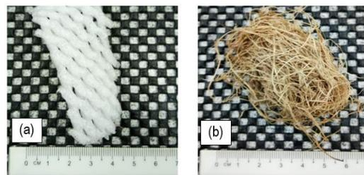
Figure 1 The solid source of (a) fruit cover plastic waste, and (b) oil palm fibre
