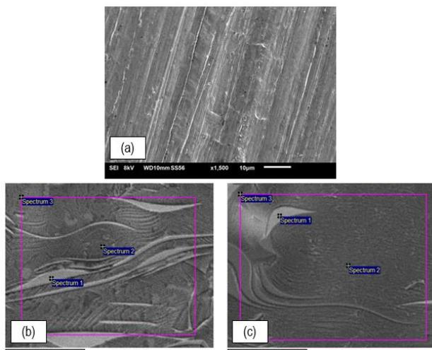
Figure 5 The SEM image of (a) a pure copper, (b) carbon grown from fruit cover plastic waste source, and (c) oil palm fibre source
