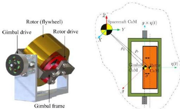
Figure 2 Control moment gyroscope (CMG).
