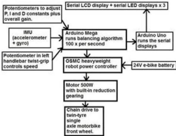
Figure 1 An example of main components of self-balancing control system.
