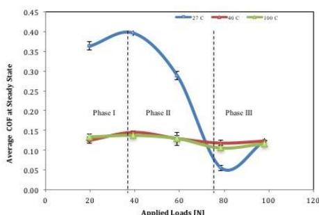
Figure 1 Average COF at steady state different applied loads [N] for operating temperatures of 27, 40 and 100 °C.
