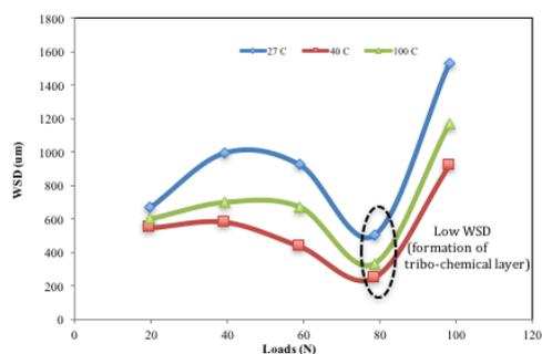
Figure 2 WSD ( $\mu\text{m}$ ) at various loads and temperatures.
