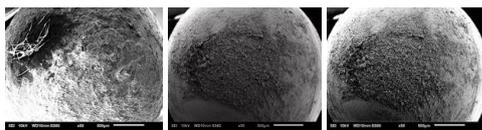
Figure 3 SEM micrograph of monolayer of tribo-chemical film at the hemisphere surface of the pins at a) 27°C, b) 40°C and c) 100°C respectively.
