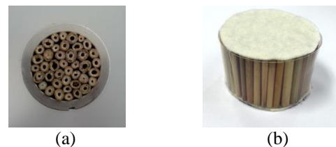
Figure 1 Sample of reed (a) in axial arrangement and (b) with attachment of felt fabric.
