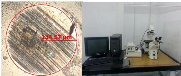
Figure 1 Sample of measured WSD of RG and SEM.
