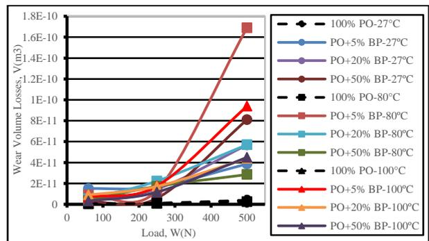
Figure 3 Effect of load on wear volume losses
