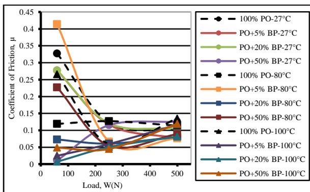
Figure 2 Effect of load on coefficient of friction.
