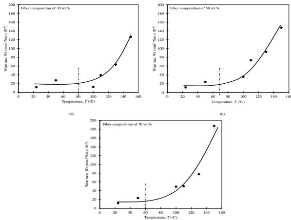
Figure 1 Effect of temperature on the wear rate of OPF/E composite (a) 30 wt.% (b) 50 wt.% (c) 70 wt.%.
