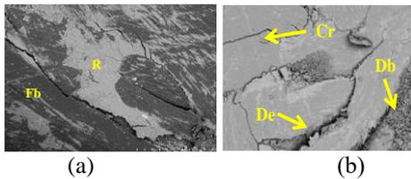
Figure 2 SEM micrographs of worn surface of 30wt.% OPF/E composite at (a)50°C and (b)130°C [De: debonding, Db: Debris, Fr: Small fracture, Cr: Micro-Crack, R: Resin. Fb: Fiber].
