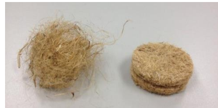
Figure 1 Raw kenaf fiber (left) and layers of kenaf fiber forming a sample with thickness of 10 mm (right).
