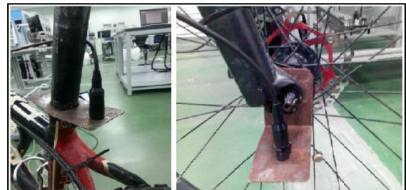
Figure 2 Accelerometer placement: Seat post (left) and front fork (right).
