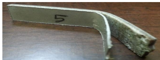
Figure 4 Failure mechanism of OPC FML
