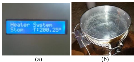
Figure 5 (a) Temperature display in R6 system; (b) Cooking pot equipped with ceramic band heater
