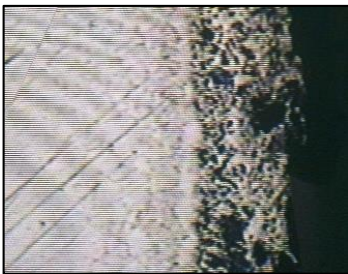
Figure 5 Cross-section of boronized 316 stainless-steel ball bearing with parameters 950 °C, 2 hours, 10 mm powder surrounding and 100 % powder concentration.
